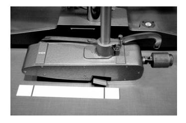
**2.6.** Place the Pendulum Arm in its release position. The Tester is now set ready for operation.
