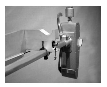
2.3 Correct the zero setting as necessary by adjustment of the Knurled Friction Rings "G". If the Pointer has swung past the zero position, Friction Rings "G" are screwed up a little more tightly. If it has not reached zero the Knurled Friction Rings "G" should be unscrewed a little. Repeat this procedure until three consecutive zero readings are obtained. Note: There are two Knurled Friction Rings; the outer Friction Ring must be unlocked before the inner Friction Ring can be adjusted.
