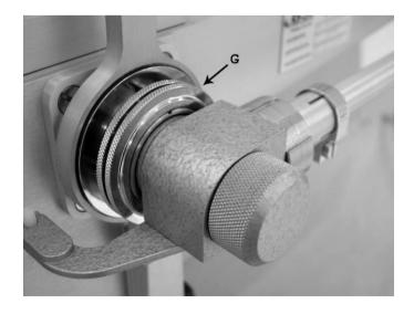
2.4. With the Pendulum Arm free and hanging vertically, place the Spacer, which will be found attached by a chain to the Base Rear Leg, under the Lifting Handle Setting-Screw to raise the Rubber Slider. Unclamp the Locking Knob "D" and lower the Head Unit of the Tester using Vertical Movement Control Knobs "E", until the Rubber Slider just touches the test surface across its width, then clamp in position with Locking Knob "D". Remove the Spacer. The approximate sliding length has now been set.
