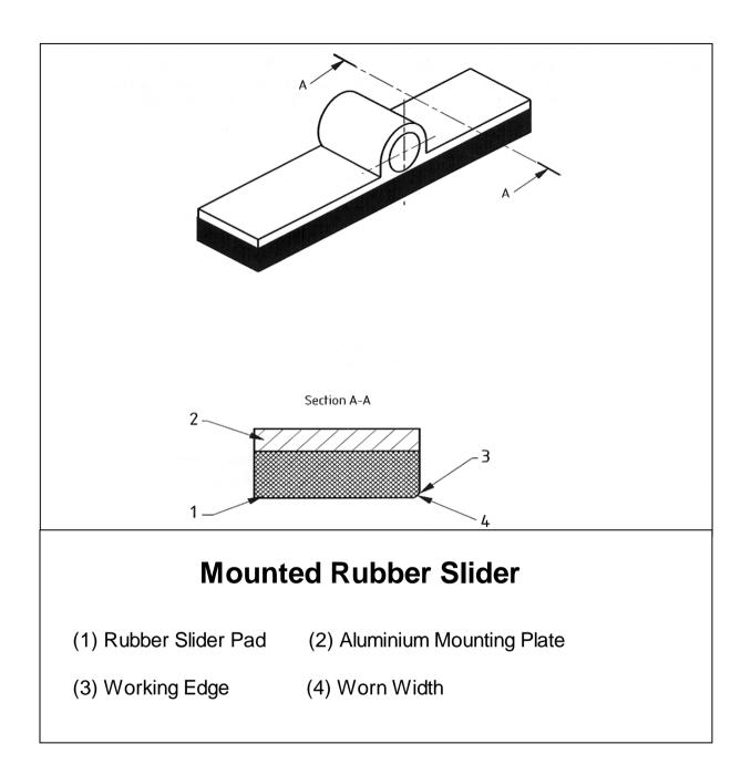
Note: When the width of the working edge of the Rubber Slider exceeds 4mm, this edge shall no longer be used. The edge should be suitably disfigured to prevent its further use. Once both working edges have exceeded 4mm the Rubber Slider should be discarded.
