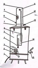
2. Put on power supply, the red light comes on, evaporation pan water level is less than level probe light yellow when the water reaches a level detector probe when yellow lights, lights, heating elements began to work.
